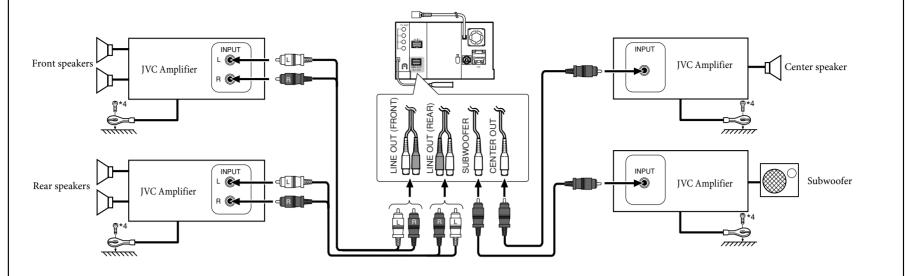
Firmly attach the ground wire to the metallic body or to the chassis of the car-to the place uncoated with paint (if coated with paint, remove the paint before attaching the wire). Failure to do so may cause damage to the unit.
